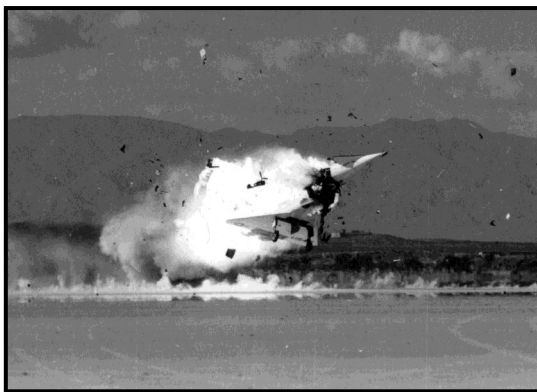
Not all test flights went as planned. The first flight of the third X-10 came to brief end due to the destruct package being mistakenly wired to the landing gear retraction switch.
