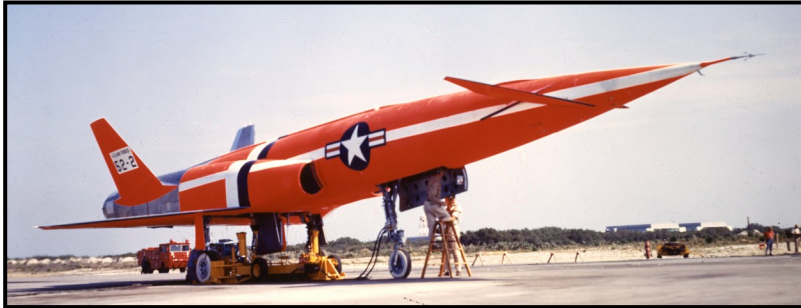
All of the X-10 aircraft that flew from Cape Canaveral Missile Test Center bore a colorful paint scheme to assist with long range tracking. This X-10 Navaho, number 52-2, was lost at sea on its first flight out of the Florida test center.
