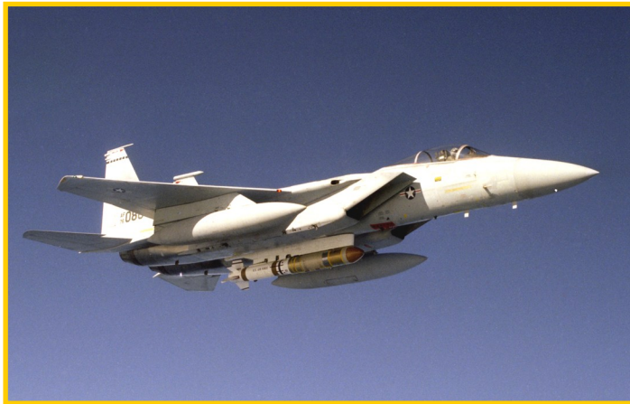
A Ling Temco Vought ASM-135 ASAT missile beneath F-15A Eagle, 76-0086 during a test flight out of Edwards AFB, CA.
