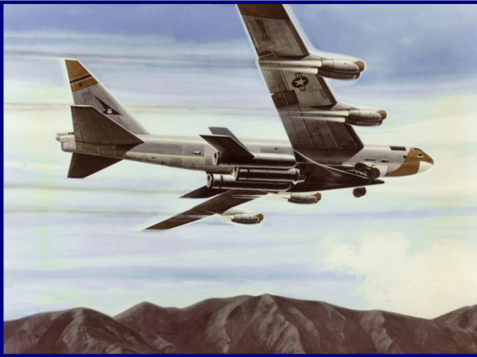
Initial flight testing of the Dyna-Soar had the vehicle dropped from a modified B-52C, 53-0399, carrier aircraft to test atmospheric handling qualities and landing techniques. The USAF selected Edwards AFB, CA, and White Sands Missile Range, NM, due to their natural runway surfaces. (AFTC History Office)
