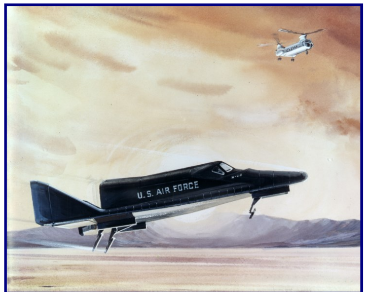
With a safety chase helicopter hovering in the background, a USAF X-20 Dyna-Soar comes in for a landing on the natural dry lakebed at Edwards AFB, CA. Due to extreme temperatures during reentry, Dyna-Soar used skids in place of conventional wheeled landing gear. (Boeing Historical Archives)
