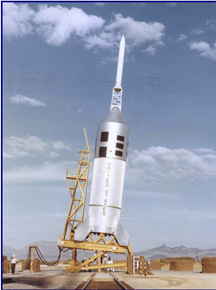
The Little Joe II was a workhorse of the early Mercury and Apollo space programs. Spacecraft escape, and parachute recovery systems were extensively tested using the reliable booster (above, left). Artist concept of Little Joe II/Dyna-Soar concept (above, right). (NASA- above, left; Convair-above, right)
