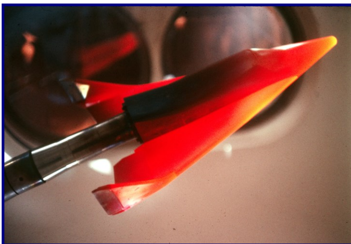
The effects of aerodynamic heating show up well on this model of Dyna-Soar during a 1962 test in the von Karman Facility (VKF) at Arnold Engineering Development Center, TN. (AEDC History Office)
