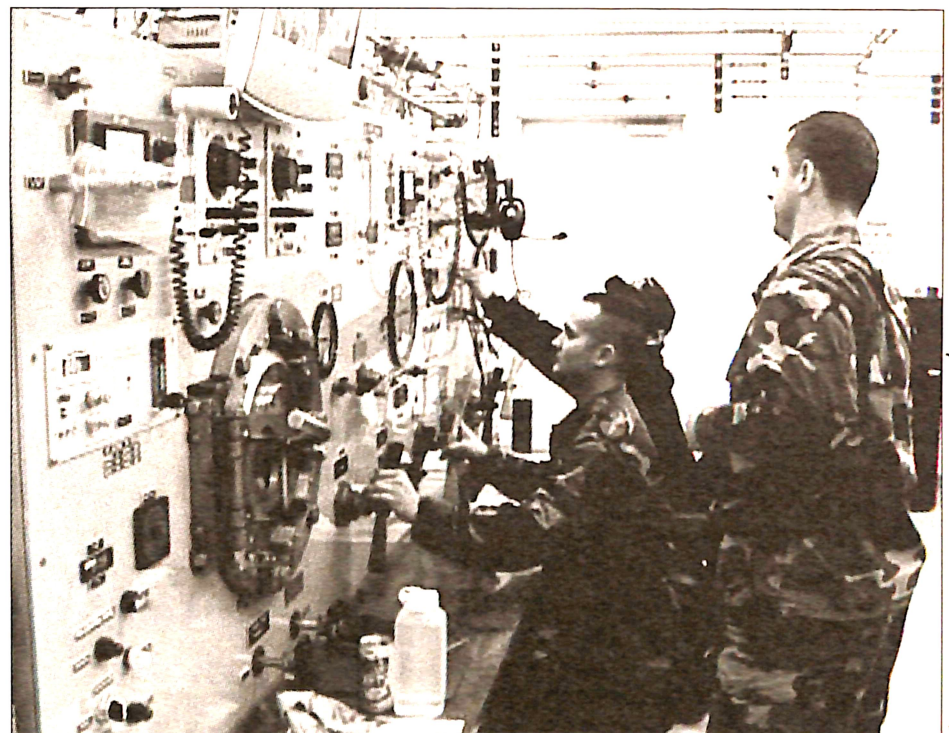
(Pictured above at left) A Patient is brought into the recompression chamber and given 100 percent oxygen through a mask. (Directly above) Divers operate the recompression chamber for the hypobaric oxygen treatment at Ship Repair Facility and Japan Regional Maintenance Center's Dive Locker.
