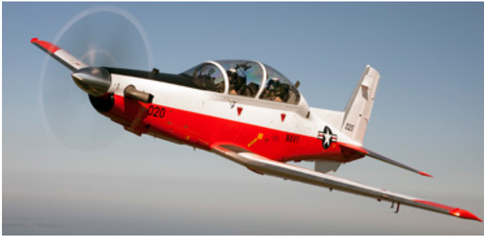
The T-6B Texan II, built by Textron Corporation, is a tandem-seat, turboprop trainer whose mission is to train Navy and Marine Corps pilots and flight officers. USNTPS has been flying the Texan II since 2010.
