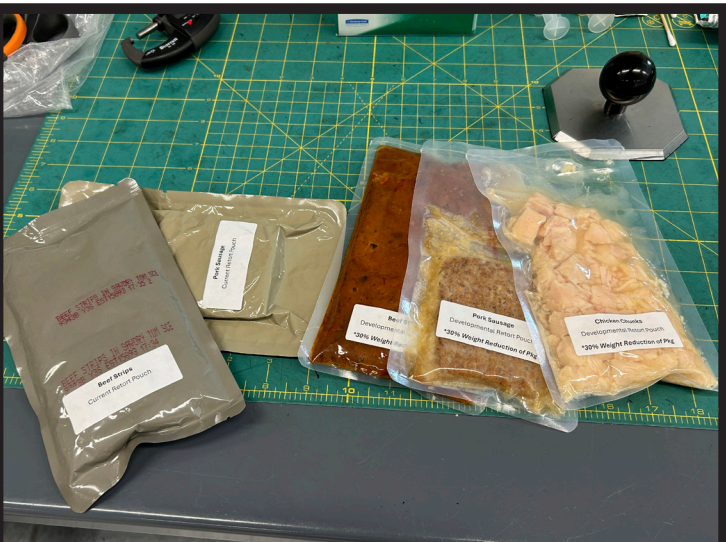
At the Army Combat Capabilities Development Command Soldier Center in Natick, Mass., packaging is engineered to allow very little water and oxygen to permeate its barriers, helping to preserve food longer and keep it safe from potential contaminants. (Photo by Katie Lange, Pentagon News)
