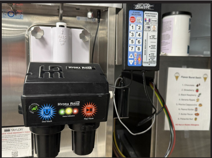
The Navy lab at the Army Combat Capabilities Development Command Soldier Center’s Combat Feeding Division in Natick, Mass., July 7, 2025, is experimenting with a fully automated cleaning system to attach to ice cream machines already on aircraft carriers, cutting the time and personnel required to manually clean each machine. (Photo by Katie Lange, DOW)
