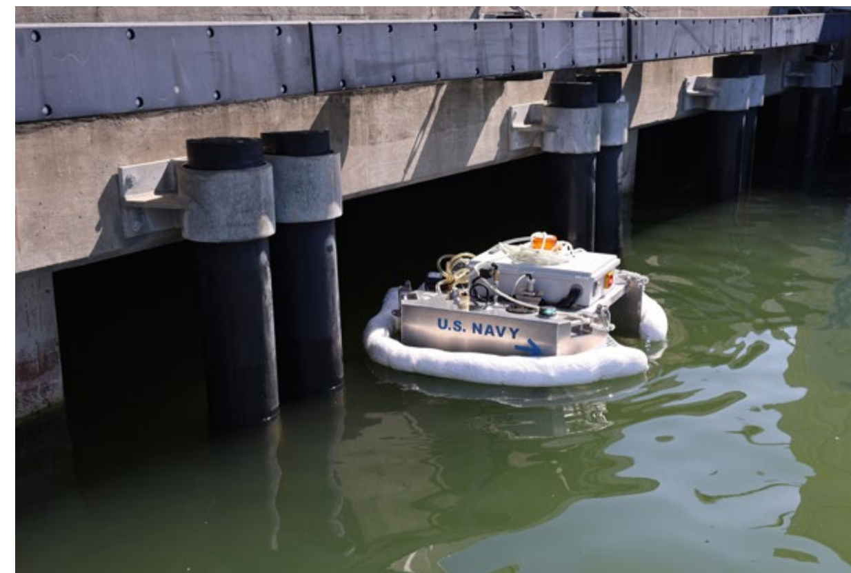
During a training exercise, NAVFAC Mid-Atlantic Environmental Oil Recovery team members practice maneuvering the Remote-Control Skimmer under a pier at Naval Station Norfolk to demonstrate the vessel's adaptability to various conditions.
