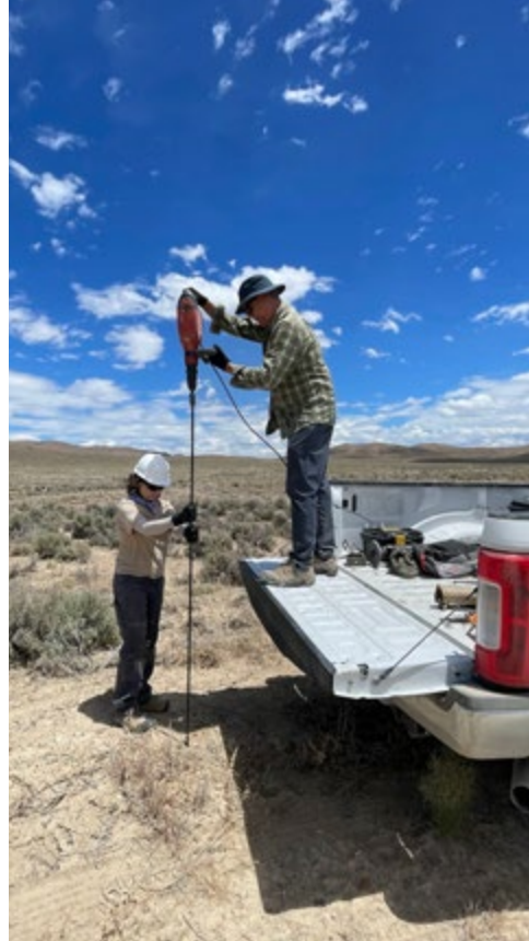
Geothermal Program Office team members install 2-meter temperature probes in the ground near the Naval Air Station Fallon ranges in Nevada, as part of geothermal exploration efforts for the Department of Energy-funded BRIDGE project.
