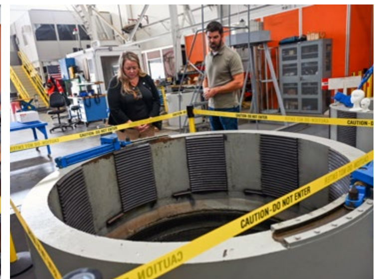
Oceans Technical Department Business Manager Paul Oemisch describes the Deep Ocean Simulation Facility, which has two chambers that enable in-water functional tests of undersea equipment at ocean pressures ranging from just below surface to a maximum depth of 34,000 feet.
