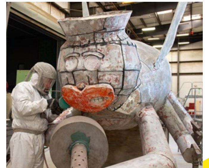
Michael Holguin, Work Leader at the Expeditionary Maintenance Center, sands around the Fighting Seabee’s mouth to remove layers of cracked paint and filler while restoring the statue’s character.
