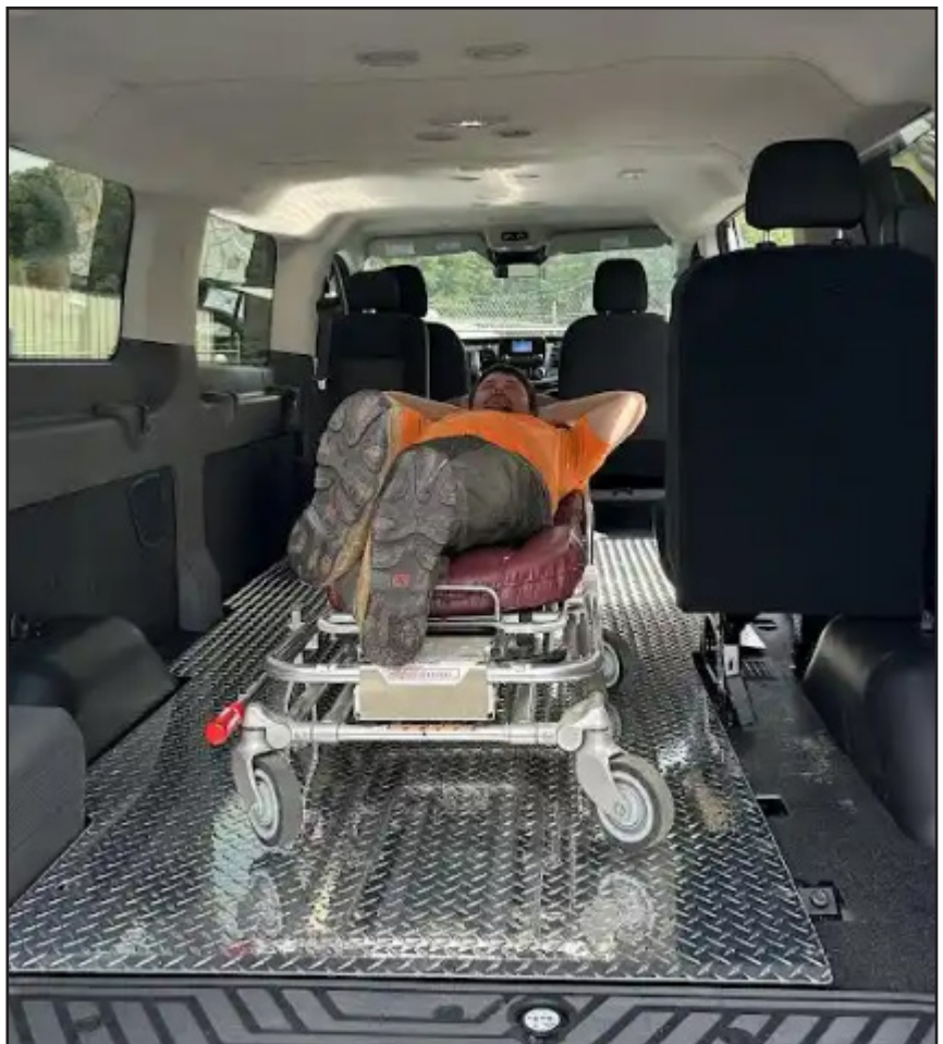
Pine Bluff Arsenal's Directorate of Public Works - Sheet Metal Shop recently turned a passenger van into a one-person ambulance. The purpose of the van is to transport anyone exposed to a hazardous chemical. Spencer Silvey, on gurney, demonstrates how the van will be used. U.S. ARMY PHOTO BY CAITLIN THOMAS-DPW
