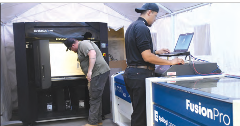
Yuma Test Center's Metrology and Simulation Division recently purchased two 3-Dimensional printers that provide a larger printing capacity and eight different materials, including carbon fiber. AJ Martin and Brendan Denney are pictured operating the largest of two printers, a Stratysys F770. (Photos by Ana Henderson)
