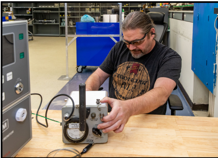
Shop 52 RADIAC Electronic Measurement Equipment Mechanic Chris Burke works on calibrating a piece of equipment with the developed 3D printed casing from Code 100TO.32, the first device developed in their partnership.
