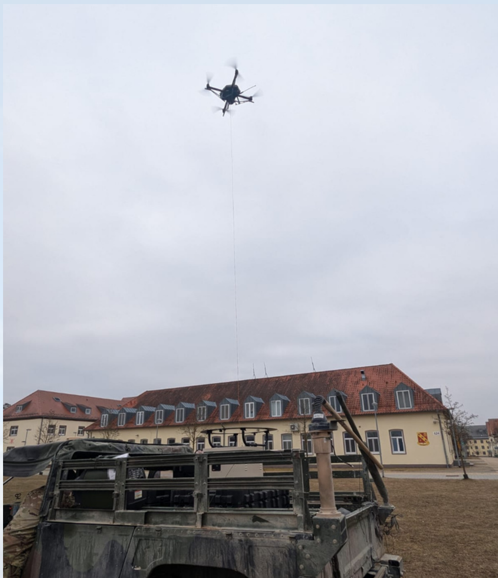
(AN UNANTICIPATED OUTPUT OF THE ACHERON CONCEPT WAS THE MOBILE VARIABLE HEIGHT ANTENNA. THE COMBINATION OF A SMALL POWER GENERATION SOURCE AND A VARIABLE HEIGHT ANTENNA MOUNTED IN A MODIFIED M1097 HMMWV ALLOWS THE RAPID DEPLOYMENT, MOVEMENT, AND EXPANSION OF COMMUNICATIONS FOR UNITS UTILIZING THE TSM WAVEFORM. THIS CONCEPT WAS VALIDATED FOLLOWING SJ24 IN GRAFENWOEHR, GERMANY.)
