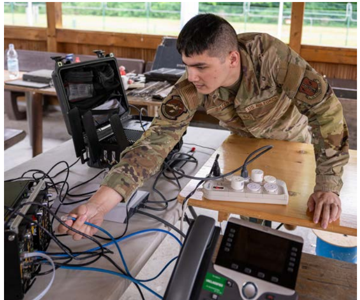
Senior Airman Dakota Gates, Client Systems Technicians, 126th Communications Flight, 126th Air Refueling Wing, Illinois Air National Guard, connects a category 5 cable to a network stack as he works to setup the AIRBUS Ranger 1200 Flyaway Satellite Communications system during an exercise at Ramstein Air Base, Germany, June 6.
