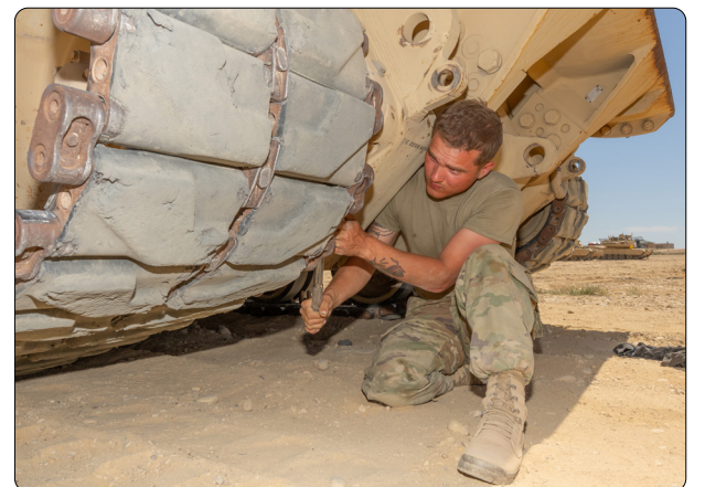
ORARNG Sgt. Philip Worthington, a mechanic with Hotel Company, 145th Brigade Support Battalion, performs track maintenance on an M88 recovery vehicle July 30, 2025, at Orchard Combat Training Center, Idaho.
