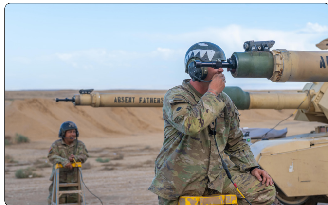
ORARNG Spc. Darren Johns and Sgt. Jose Lopez, both loaders with the 3rd Battalion, 116th Cavalry Regiment, participate in boresighting their respective M1A2SEP tanks July 28, 2025, at Orchard Combat Training Center, Idaho.
