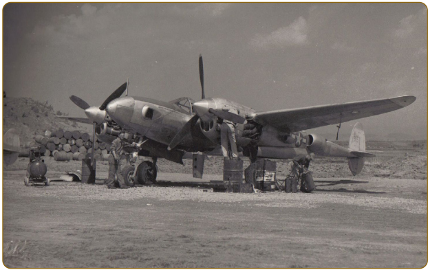
File photo courtesy of John Brasko Collection, 142nd Wing History Archive Engineering personnel of one of the detached flights of the 35th Photographic Reconnaissance Squadron are seen here servicing the engines of a Lockheed F-5E "Photo Lightning" (converted in the U.S. from Lockheed P-38J-15-LO 43-28301 to become an F-5E-2-LO, and given the squadron ID number 815) at an austere location in southeastern China late in the war. 815) at an austere location in southeastern China late in the war.
