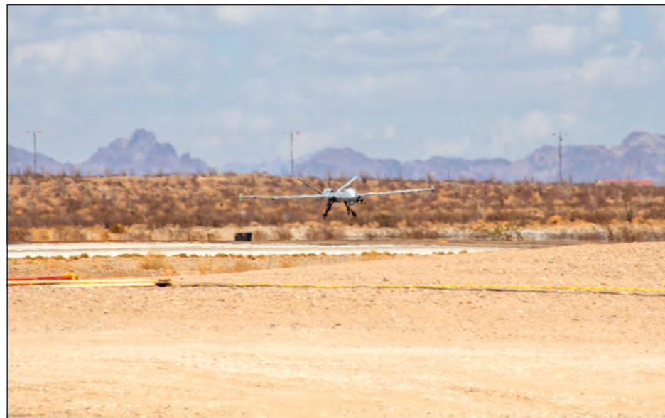
Following launch, the SB600 was maneuvered by an operator using SATCOM for over-the-horizon communication, ensuring continuous command and telemetry exchange during reconnaissance and target engagement.
