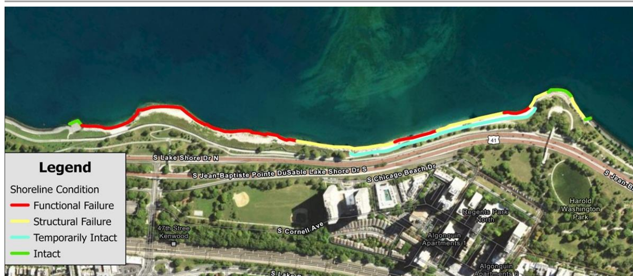
Figure 12: Coastal shoreline structure conditions indicating functional failure (2642 linear feet), structural failure (1888 linear feet) , and intact (424 linear feet) coastal protection structures. The coastal shoreline condition assessment was conducted based upon multiple site visits from 2019 – 2025, CDOT/CPK shoreline assessment reports, 2022 drone footage, Google Earth imagery, and utilizing ESRI ArcGIS mapping. (Appendix F).
