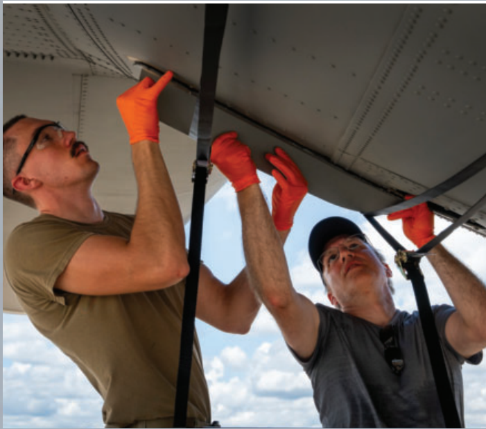
Airman 1st Class Tustin Bridges, 1st Special Operations Wing, and Bryan Jenkins, Vortex Control Technologies, install an aluminum Finlet onto the rear door of an MC-130J July 9 at Eglin Air Force Base, Florida. The 417th Flight Test Squadron's air crew and engineers will analyze the Finlets' flight and air handling qualities as well as the aircraft's airdrop compatibility with the new additions. (U.S. Air Force photo by Samuel King Jr.)
