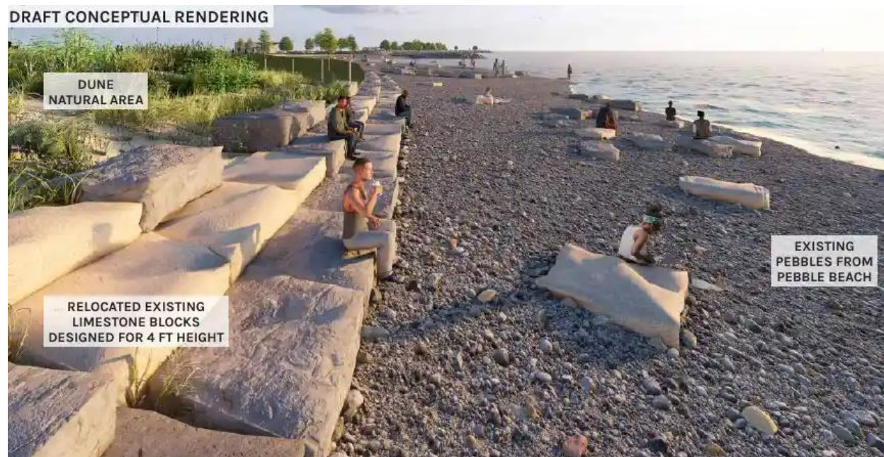
Figure 36: Draft conceptual renderings of material reuse such as backshore limestone stepped revetment, limestone seating and pebble reuse within dynamic revetment.
