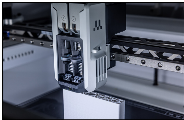
From design to print, the Innovation Lab creates a paddle prototype for Shop 36 that will be used to stir electroplating chemicals.
