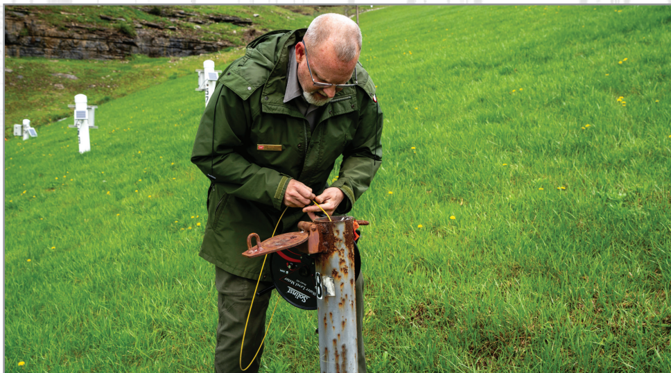
Jon Fillingham, Rough River Lake project manager, takes piezometer measurements, April 4, 2025, at Rough River Lake in Falls of Rough, Kentucky, monitoring the dam and keeping watch 24 hours a day during the high water event.
