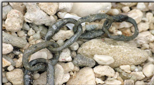
The mooring chain shows deterioration which caused it to break setting the boat adrift.
