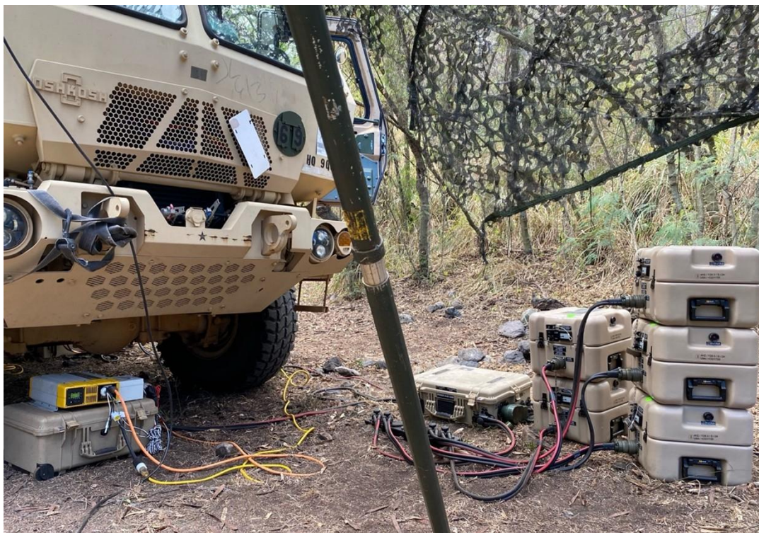
Figure 2. LMTV equipped with external energy storage solutions. 2
