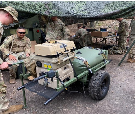
Figure 5. All Terrain Electric Cart configured for power distribution and mobile operations. 5
