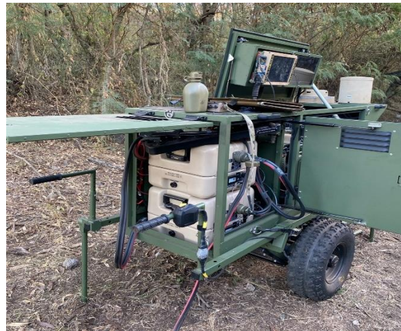
Figure 5. All Terrain Electric Cart configured for power distribution and mobile operations. 5
