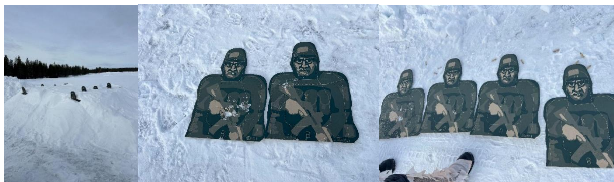
From left to right: two lane compacted snow test shoot with 240L, one meter and two-meter targets on compacted snow lane, one through four-meter targets on non-compacted snow lane.
