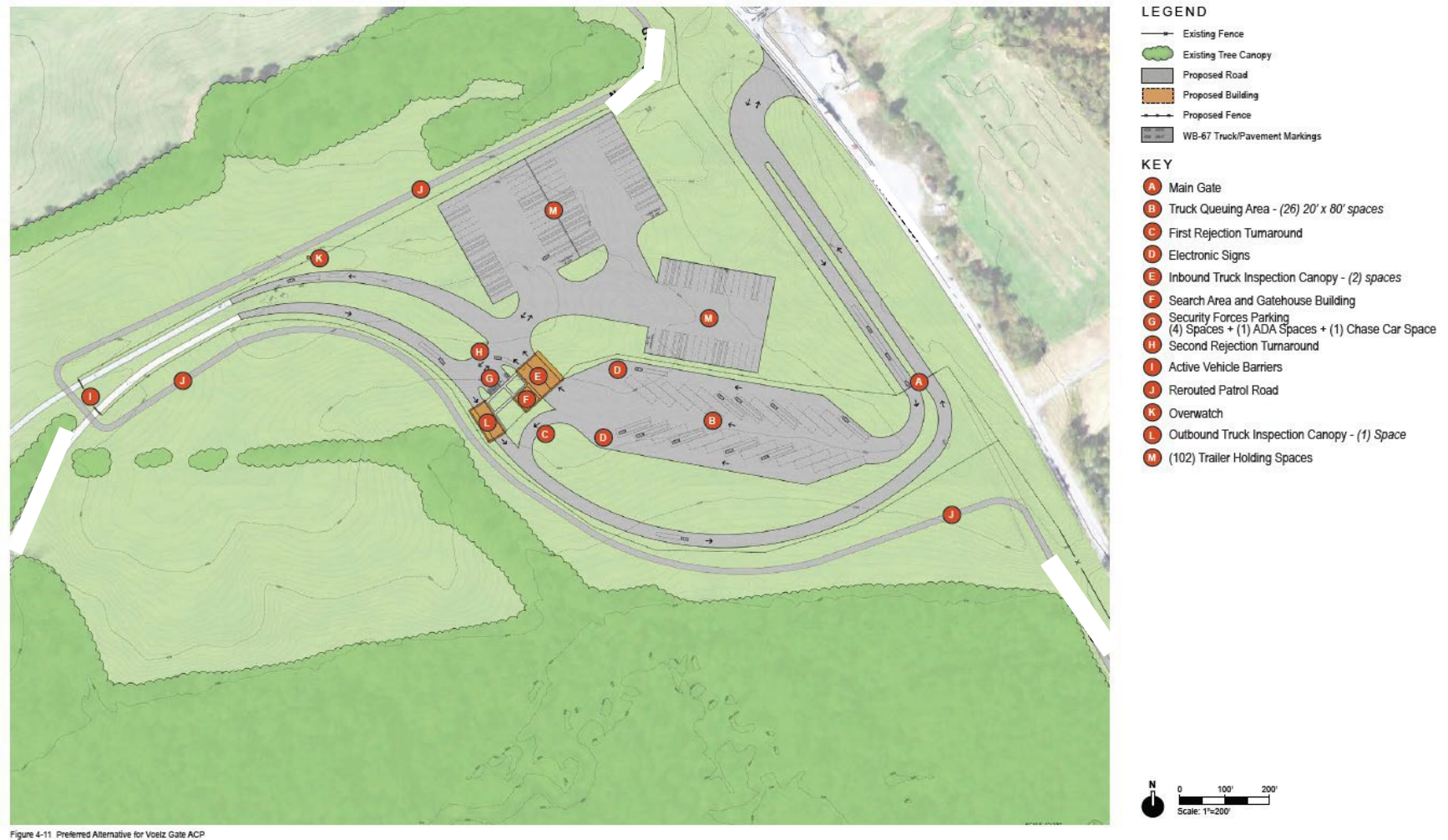
Figure 2-2: Proposed Voelz Gate ACP Design
