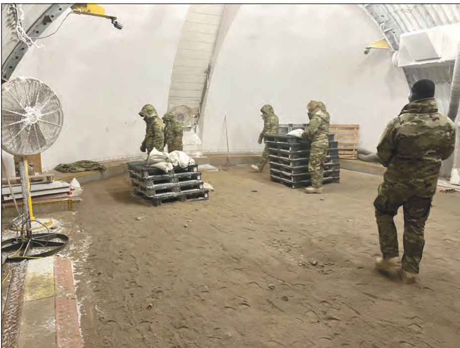
The All-Range Tactical Clothing system, formally known as the Cold Temperature and Arctic Protection System, is a multi-layer collection of cold weather garments designed to provide the wearer environmental protection in temperatures ranging from 45 °F to -65 °F. The climactic chamber at Yuma Test Center was conditioned to the test temperature prior to the start of each test day and maintained at that temperature for the duration of the day.
