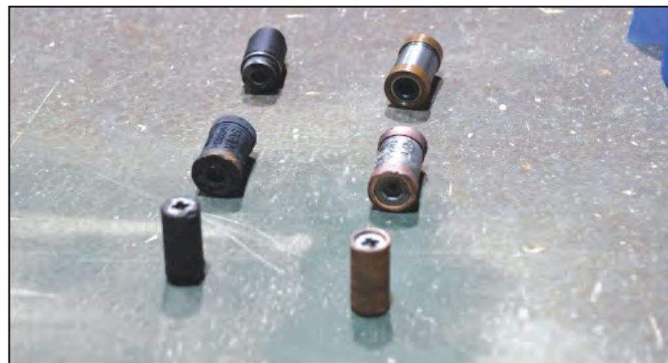
Laser Ablation Cleaning System uses laser light to remove corrosion and deposits from copper crusher gauges and other materials. The photo shows the copper crusher gauges before and after being cleaned with the system. (Photo by Ana Henderson)
