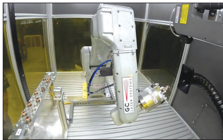
Yuma Test Center purchased a stationary Laser Ablation Cleaning System that allows for coupled and decoupled operations. In the coupled state, a robotic arm performs all the operations autonomously and in the decoupled state, personnel can decouple the laser from the robot and use it manually. (Photos by David Le)
