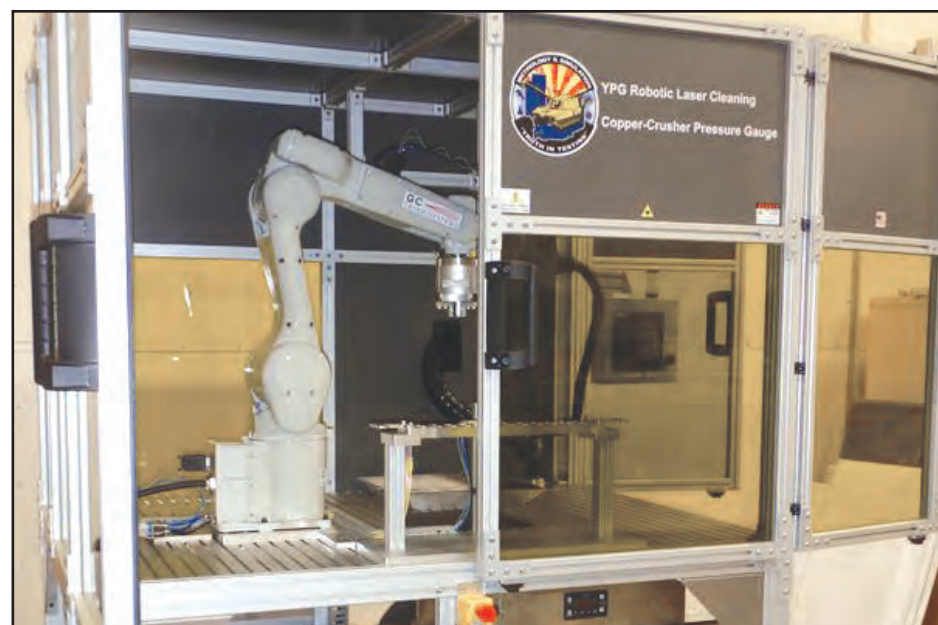
Yuma Test Center purchased a stationary Laser Ablation Cleaning System that allows for coupled and decoupled operations. In the coupled state, a robotic arm performs all the operations autonomously and in the decoupled state, personnel can decouple the laser from the robot and use it manually. (Photos by David Le)
