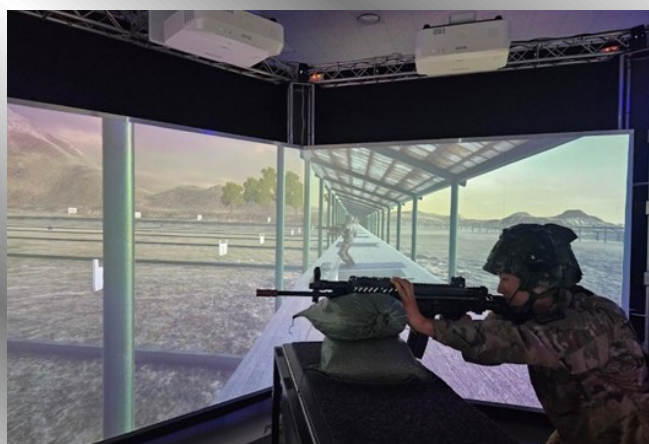
KMA utilizes sensors in the weapon and ACH to analyze missed targets.
