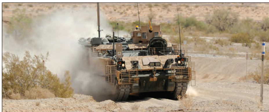
The Armored Multipurpose Vehicle underwent extensive natural environment testing at all three Yuma Proving Ground test centers. No matter how much a combat system has been tested through virtual or simulated environments, unforeseen issues arise when that system is subjected to operations in the extreme climactic conditions of arctic, tropical, or hot desert environments. (Photo by Mark Schauer)
