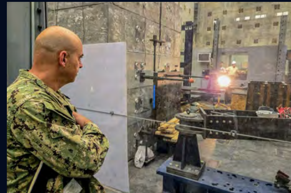
NAVFAC EXWC Commanding Officer Capt. Dean Allen inspects the test setup at Georgia Tech for a dynamic tension test of a headed rebar encased on concrete.
