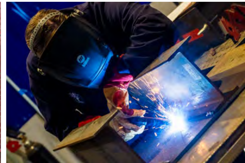
NAVFAC EXWC Engineer Thomas Erickson welds test panels in the FATHOMWERX public-private laboratory to be used for forced-entry testing.
