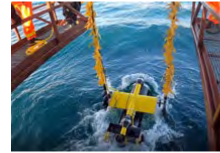
The NAVFAC EXWC team lowers a prototype Surface Towed Array Sensor System (SURTASS) into the Pacific Ocean.
