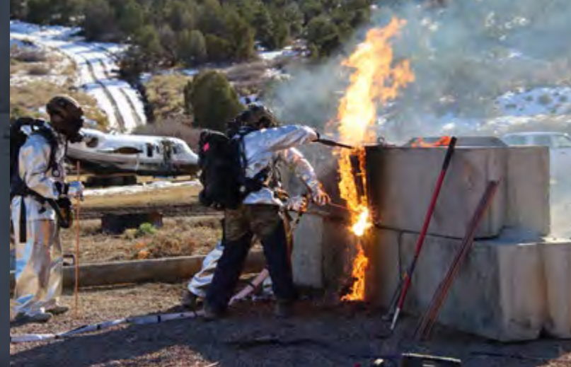
Defense Threat Reduction Agency (DTRA) special forces team members execute a combined thermal and power tool attack against NAVFAC EXWC test specimens.
