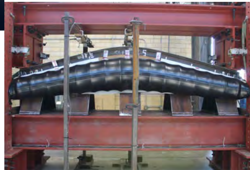
A NAVFAC EXWC test specimen is tested to failure at the University of Texas at Austin to evaluate its ability to resist the extreme forces it would experience during an explosion.
