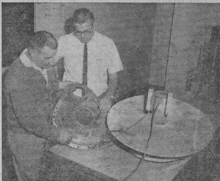
HORRIBLE EXAMPLES — Fred Novekoff, left, assistant instructor, and Dick Rosche, course administrator, look over corroded drive cover, an addition to the rogue's gallery of the Arsenal corrosion control course. Larger disc is part of corroded antenna.
