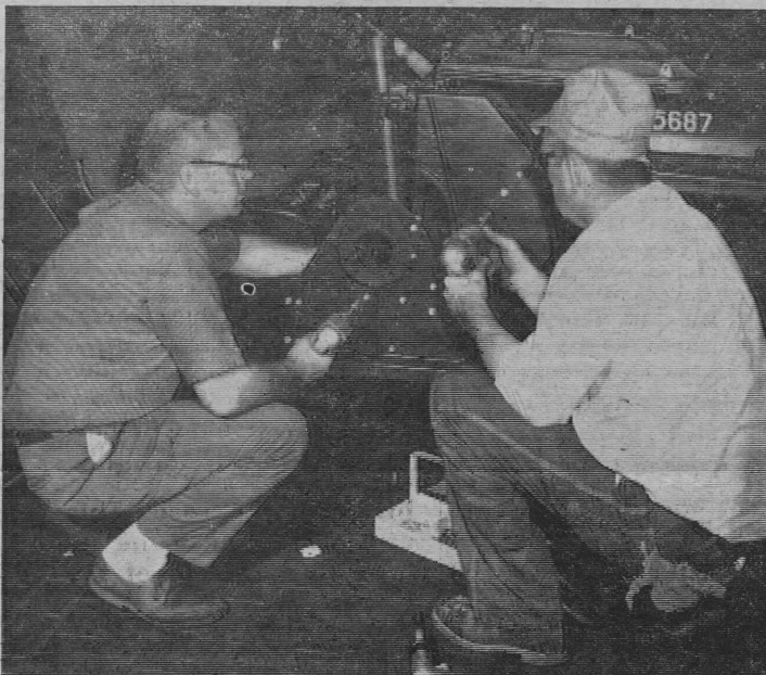
EARLY STEP — Harry Moorman demonstrates first major step in modifying jeeps — cutting away metal of standard model to make room for weapon mounting brackets. He's using pneumatic edging cutter that slices metal easily.
