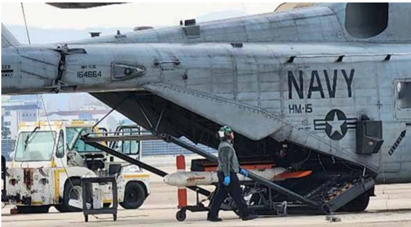
AN/AQS-24 being loaded aboard MH-53 helicopter.
