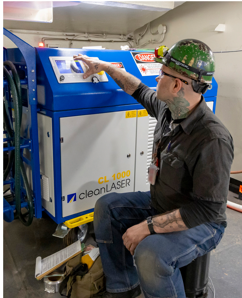
AT LEFT: Chase Absher, painter, Shop 71, Painters, Blasters, Tilessetters, adjusts the settings and parameters on the Adapt Laser CL 1000 machine, which is used to power the laser ablation tool, May 22, while working aboard USS Ronald Reagan (CVN 76).
