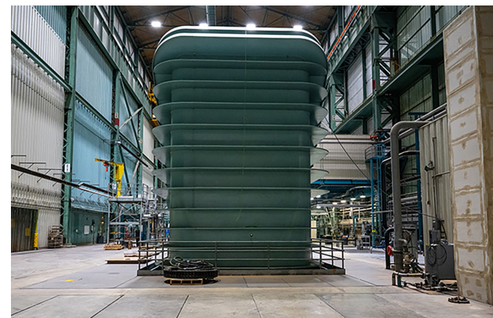
An exterior view of Naval Surface Warfare Center, Carderock Division's Large Cavitation Channel in Memphis, Tenn., on July 25, 2024. The LCC is one of the world's largest and most advanced high-speed, variable-pressure water tunnel facilities and is currently being used for cavitation erosion prevention testing. Site Director Matt Brantz led a tour of the facility as part of the Cavitation-Resistant Materials and Coating Workshop, which featured several Carderock partners from academia and government institutions.
