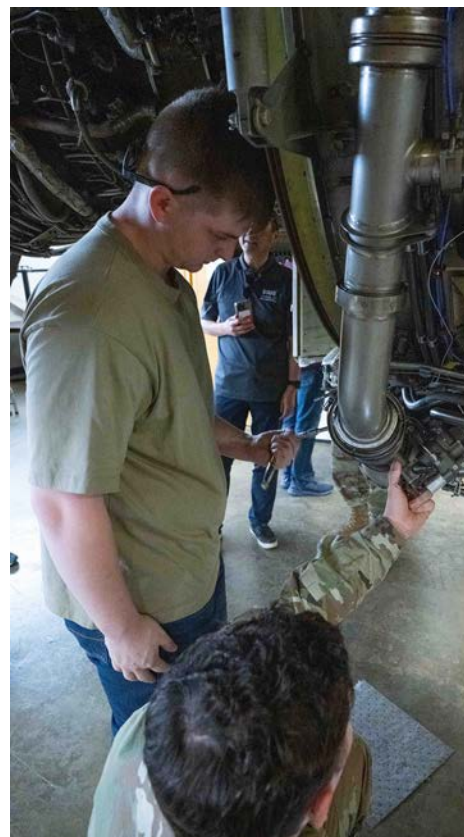
Southern Illinois University, Edwardsville, mechanical engineering student Alex Daiber, left, takes off a starter control valve, while U.S. Air Force Staff Sgt. Kyle Finsterwalder holds it in place at Scott Air Force Base, Illinois, April 22.
