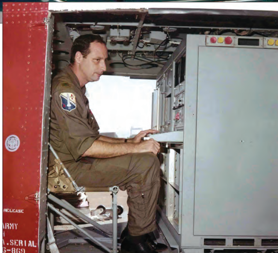
The earliest GPS systems were so large that a UH-1 helicopter, which carried as many as 14 troops at a time when used in Vietnam, could only accommodate a pilot and two passengers when carrying a GPS device. By September 1977 testers had conducted over 70 test flights with UH-1 helicopters, as seen here, and F-4, P-3, and C-141 airplanes. (U.S. Army photos)
