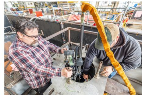
**AT LEFT:** Bryan Hara, welding instructor, Shop 26, Welders, and Josh Maya, waterfront support and welding work lead, Code 100TO.3, Moonshine Lab, install a clamp on the BOA-550 Welding Machine, April 9, in Building 460 at PSNS & IMF.
