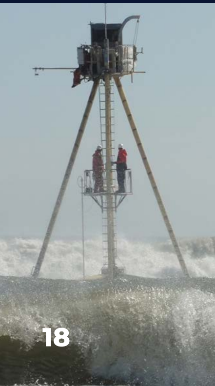
R&D Facilities supports data collection with the Coastal Research Amphibious Buggy (CRAB).
