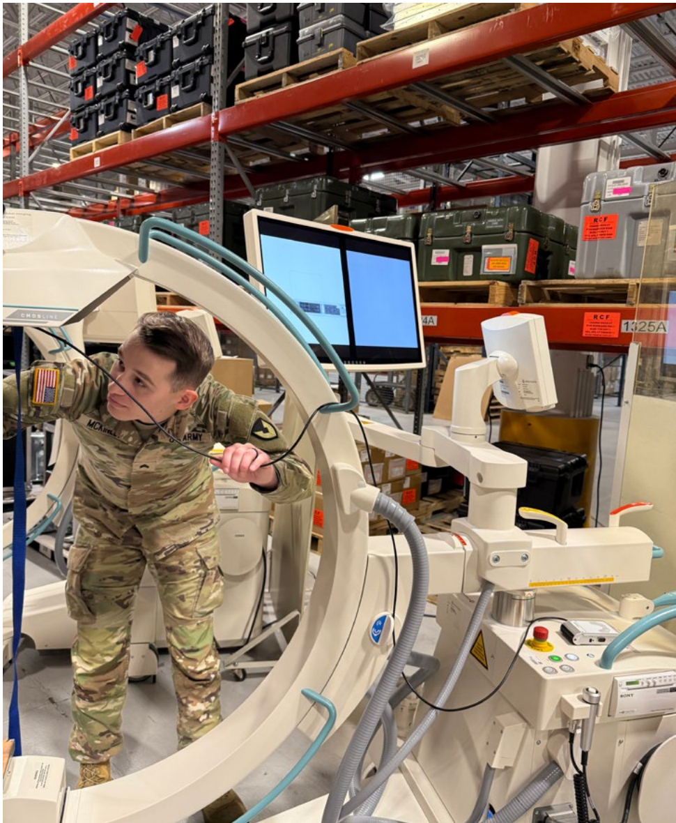
Sgt. Nicholas McKinley, a biomedical equipment specialist, inspects a C-Arm machine, a mobile imaging device that uses X-rays to provide real-time images during surgical procedures, at the U.S. Army Medical Materiel Agency's Medical Maintenance Operations Division at Hill Air Force Base, Utah. While medical maintenance is McKinley's regular job, he also recently joined the Army Esports Team, competing as a member of the World of Warcraft dungeons team. (U.S. Army photo by Staff Sgt. Nora Martinez/Released)
