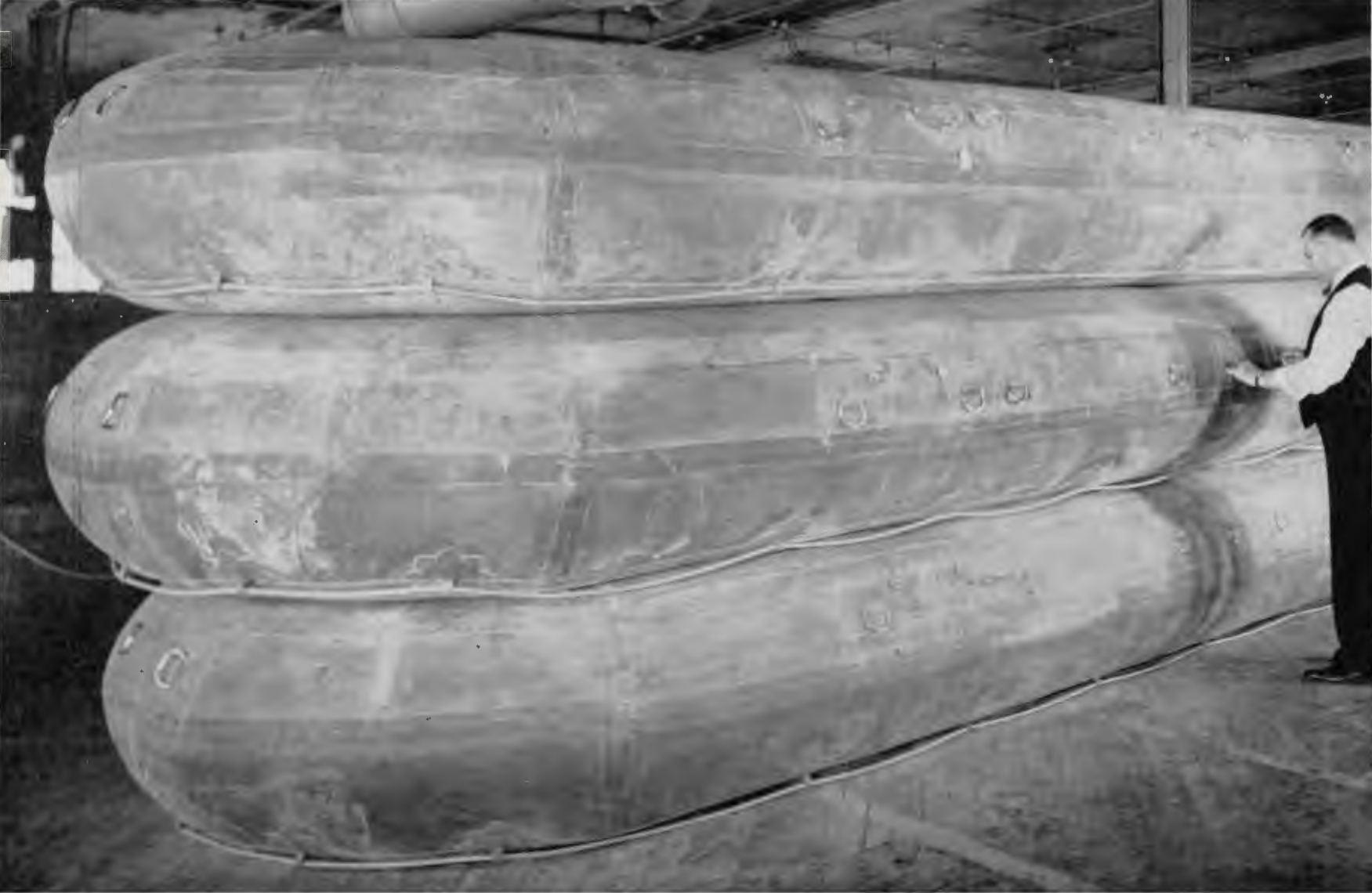
Pneumatic floats (pontoons) are made of rubber and fabric. Made into bridges they can bear the weight of a 28-ton tank. Deflated, they can be made into o
