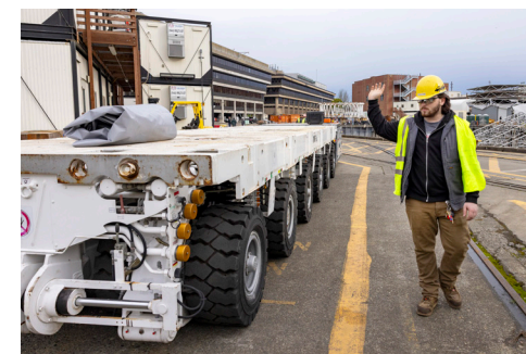
ABOVE: A team of Code 740, Riggers, maneuvers a self-propelled modular transport along Farragut Avenue Feb. 21, before delivering it to Dry Dock 5.
