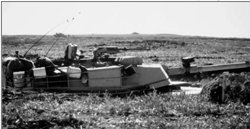
Hull defilade position for an M1 tank.
