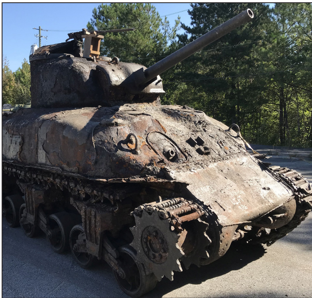
The introduction of the M4A1 “Duplex Drive” Sherman tank, like this one recovered off the Normandy beach, was designed to enable infantry forces to storm the beaches as part of the Allied invasion, unfortunately 27 of the 29 tanks deployed sank before they reached landfall.
