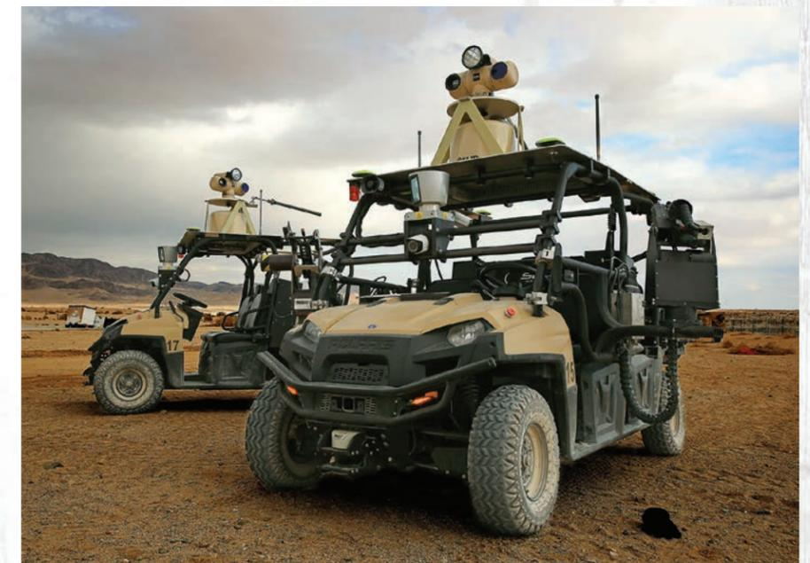
A Mobile Detection Assessment Response System is used during a CERDEC-Technology Enhancements in Autonomous Machines, or C-TEAM, Robotics Demonstration at Range 1, Joint Base McGuire-Dix-Lakehurst, New Jersey. (U.S. Army photo)
