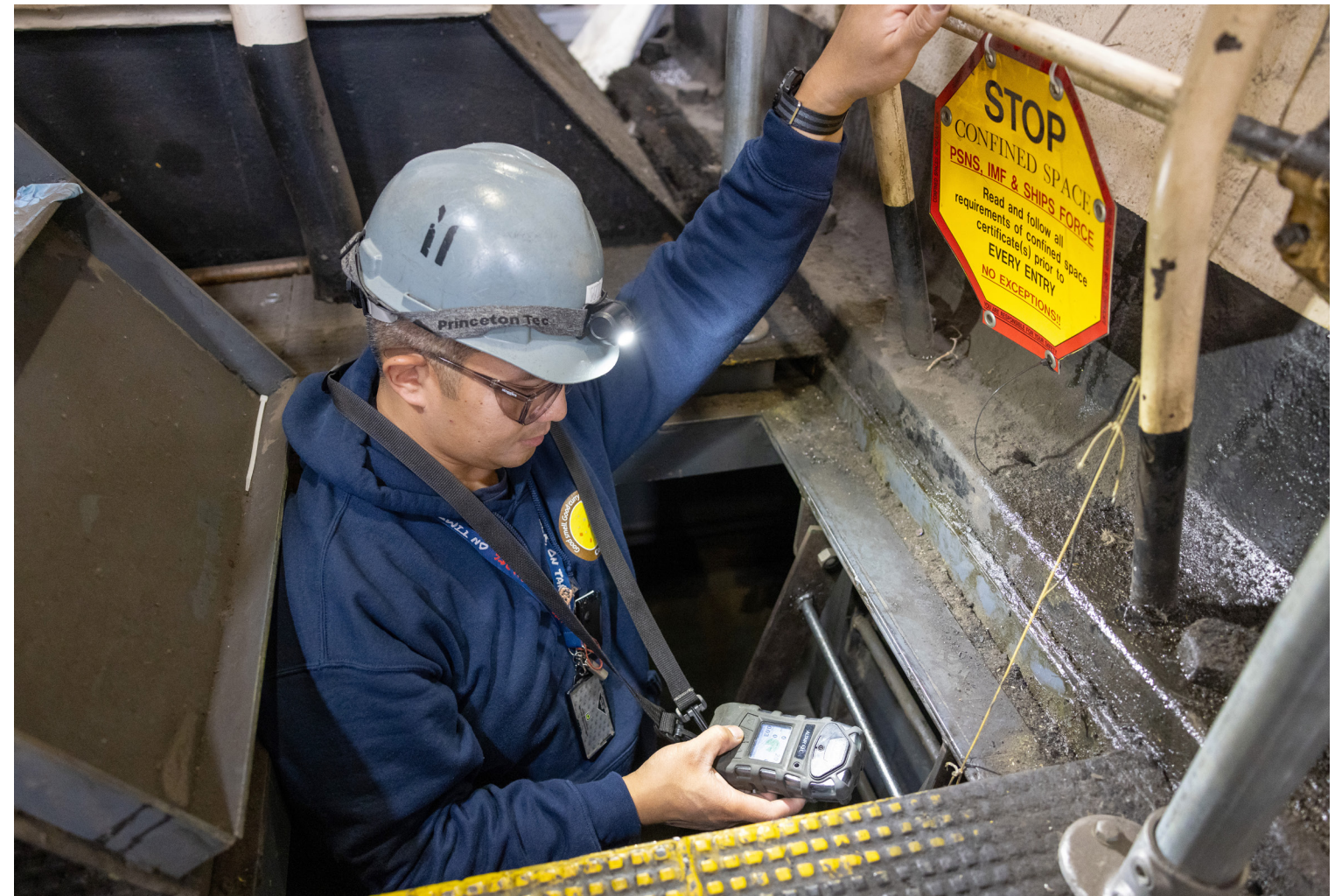
ABOVE: Michael Galvez, shipfitter worklead, Navy competent person, Shop 11, Shipfitters Gas Free, works inside the roller pit of a large flange turning machine, Oct. 18, while completing a gas-free inspection in Building 460 at PSNS & IMF. (U.S. Navy photo by Wendy Hallmark)
