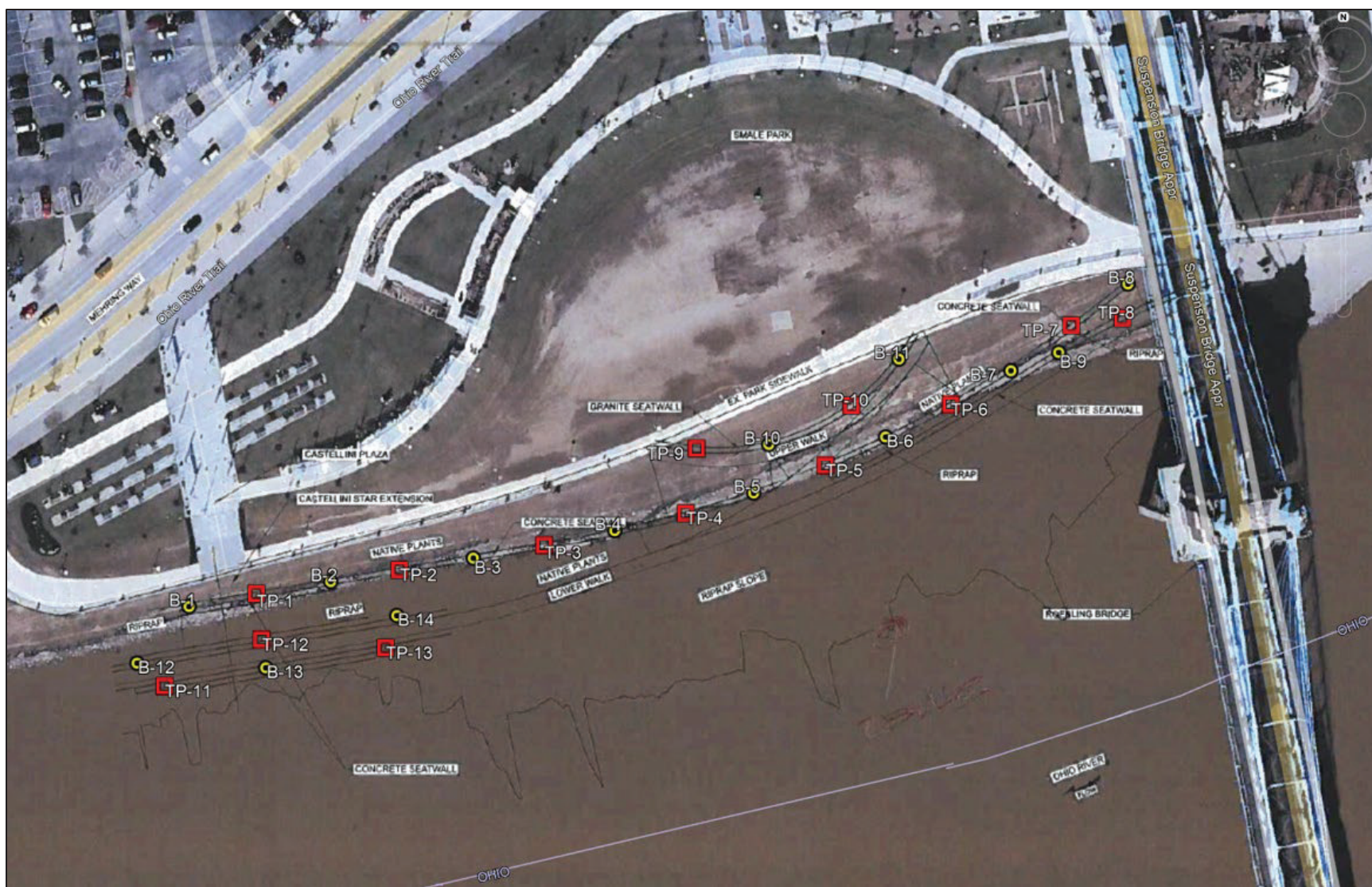
Figure 2: Aerial overview of the of the proposed locations of the geotechnical backhoe trenches (red rectangles) and soil borings (yellow circles) within the APE.
