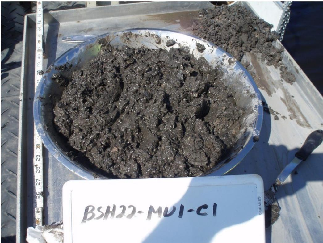
Figure 16: MU1-C1 composited and homogenized sample
