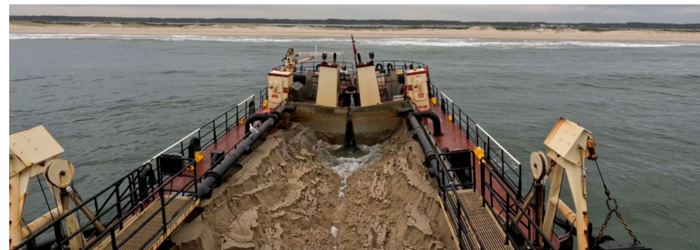
The MURDEN can transport roughly 50 dump trucks worth of material and deposit it in the surf zone to nourish sand-starved beaches. (U.S. Army Corps of Engineers photos by David Adams)
