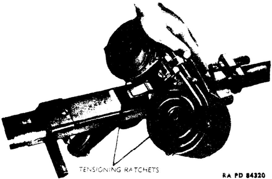
**Figure 27 — Mounting of 75-round Magazine**
