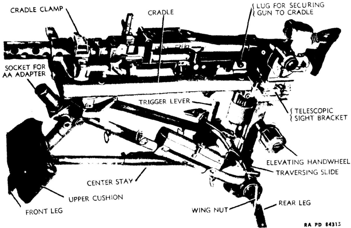
Figure 5 Machine Gun — on Tripod Mount
