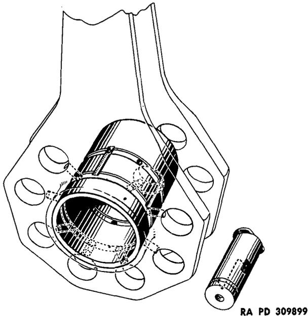
Figure 86 – Master Rod and Bearing
