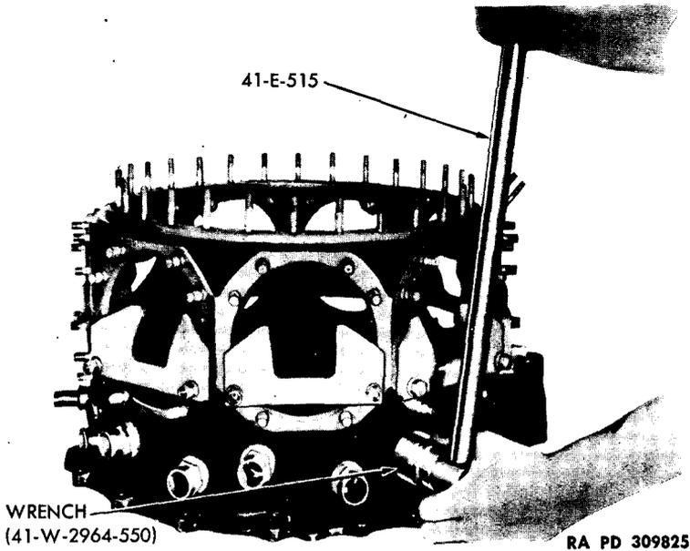
**Figure 90 — Removing Valve Tappet Retainer Nut**
