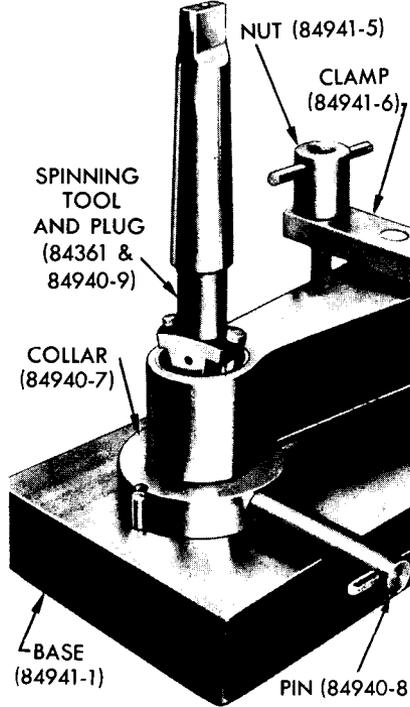
**D—SPINNING OVER ENDS OF BUSHING**
