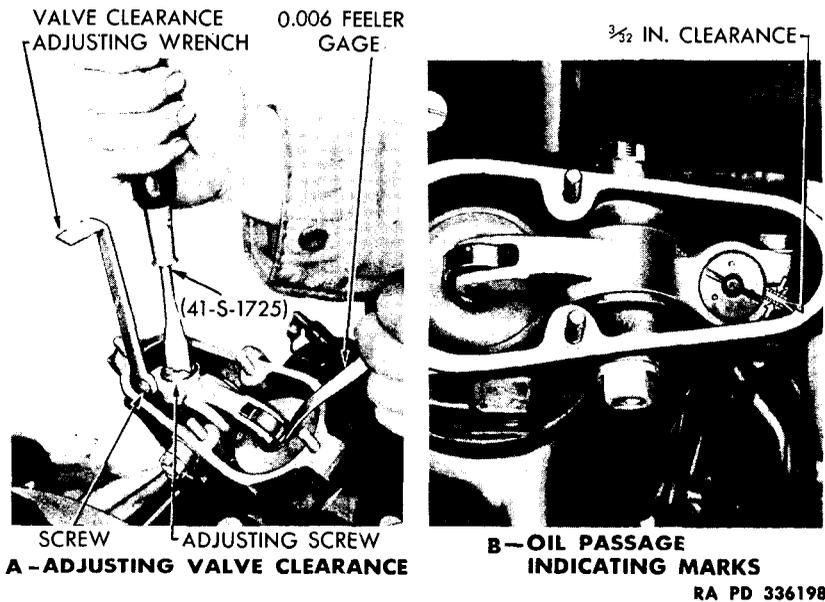
**Figure 148 — Adjusting Valve Clearance (Previous to Engine No. 305029)**
