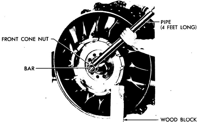
2. TIGHTENING FRONT CONE NUT
