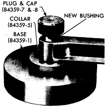
B — INSTALLING NEW BUSHING
