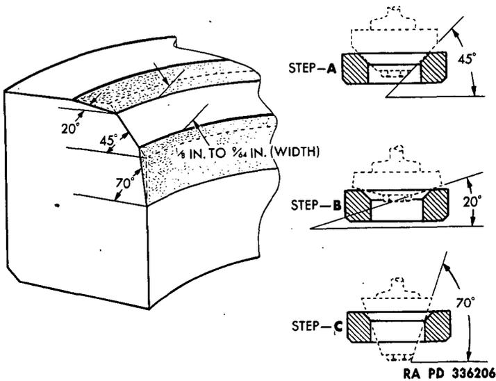
**Figure 81 – Valve Seat Insert Angles for Reconditioning**
