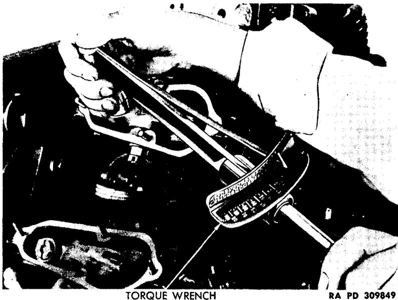
**Figure 149 — Tightening Tappet Adjusting Screw Lock Nut**
