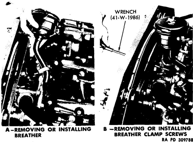
*Figure 25 - Removing Atmospheric Breather*
