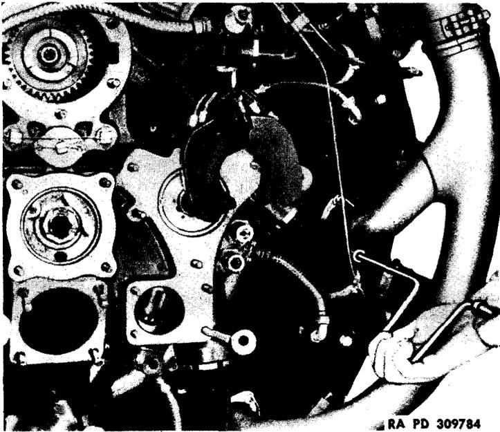
**Figure 16 — Removing Exhaust Manifolds**
