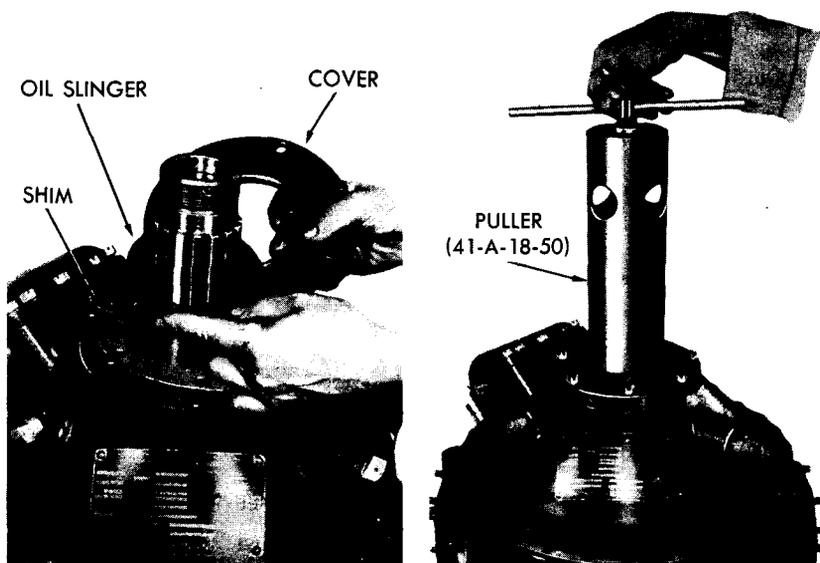
A—REMOVING OR INSTALLING
