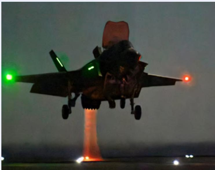
*U.S. Marine Corps test pilot Maj. Paul Gucwa performs a vertical landing (VL) in an F-35B Lightning II. Gucwa also performed the first night shipborne rolling vertical landing (SRVL) during the evening's flight period.*
