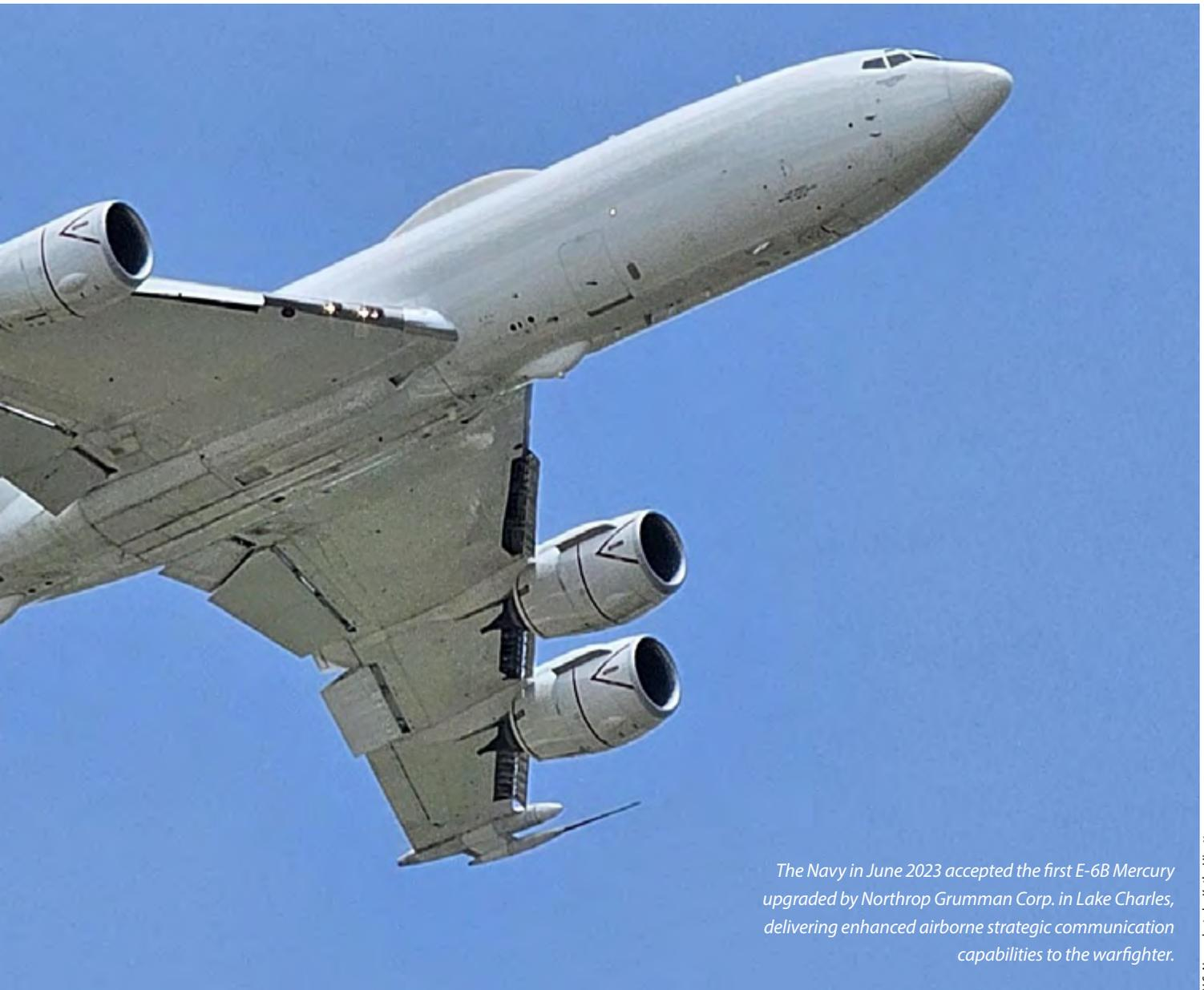
*The Navy in June 2023 accepted the first E-6B Mercury upgraded by Northrop Grumman Corp. in Lake Charles, delivering enhanced airborne strategic communication capabilities to the warfighter.*
