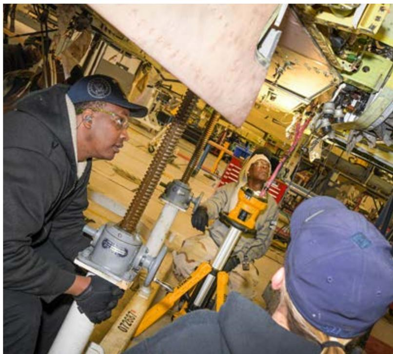
*Artisans assigned to Fleet Readiness Center Southeast's F-5 Production Line prepare to remove the wing of an F-5N Tiger II aircraft for inspection.*
